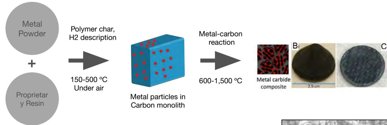
Synthesis process for Nanoarmor UHTCMCs (above) and the resulting homogenous microstructure (right) without any additional densification steps
