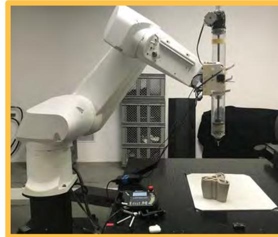
**Nanoarmor ZrC has been successfully extruded into complex near-net shape parts via additive manufacturing processes**
